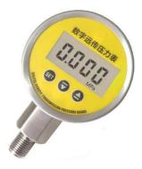
Digital Remote transmission Pressure Gauge has LED or LCD display with 4-Digits, display digits are optional too. There are 3 buttons on front panel set up the gauge. It is easy to install in Pipeline, Isolation Tank or others connects device, easy to set up operating parameter. Working condition is -20~80 °C.
