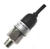
XY-PS700B Mechanical Pressure switch, Upright type, work only by mechanical deformation, No power supply needed for switching of electrical loads, when the force impact on the pressure-sensitive components to make mechanical deformation, the pressure switch will move up through the mechanical structure such as balustrade spring and finally trigger the micro switch at the top, then output electrical signals.
